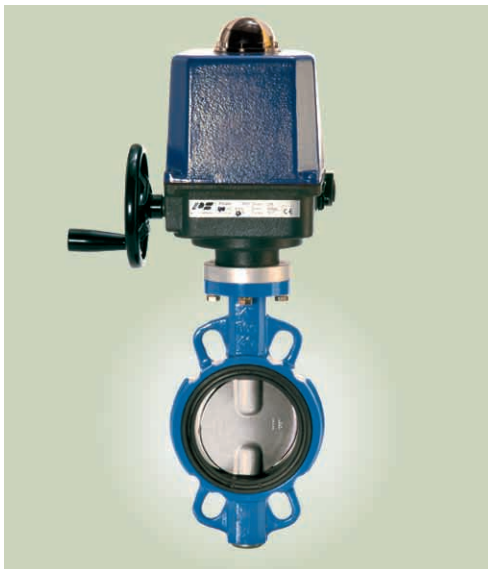
VALVOLA A FARFALLA con attuatore elettrico monofase 230V - 50HZ o trifase 400V - 50HZ IP67. BUTTERFLY VALVE with 230V - 50HZ one phase or 400V - 50HZ three phases IP67 electric actuator.
